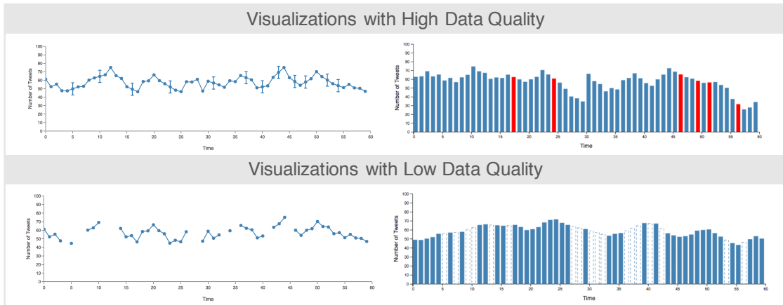
Fig. 1: We measured factors influencing response accuracy, data quality, and confidence in interpretation for time series data with missing values. We found that visualizations that highlight missing values have higher perceived data quality while those that break visual continuity decrease these perceptions and can bias interpretation.
