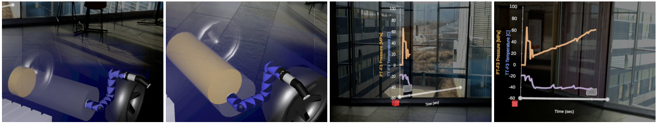
Figure 5: Simulated hydrogen fuel fill-up. As time elapses, simulated hydrogen flows into the tank (a,b) and the Temperature-Pressure profile of an average fill populates in real-time (c,d).
